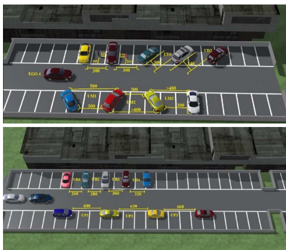
Fig. 10 Multiple scenarios set-up for benchmarking. The testing area is the parking zone of Panasonic Europe (Langen, Germany). Due to General Data Protection Regulation (GDPR) law, no real picture can be shown, but the simulated picture is very close to the real one.
