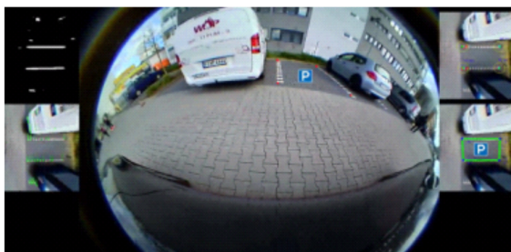
Fig. 7 Example of park-marking detection projected in both perspective view and top-view on the sides. White dashed park-marking is detected and displayed with "P" mark.
